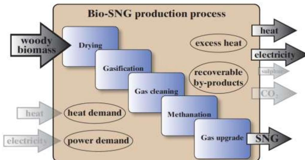
**Figure 1: BIO-SNG PRODUCTION PROCESS**
